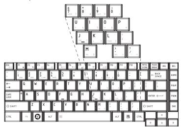
Figure 5-1 The numeric keypad overlay
