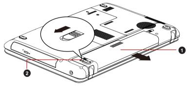
2. Battery release latch Figure 6-2 Releasing the battery pack - 2
