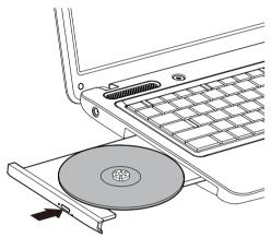
Figure 4-5 Closing the disc tray
