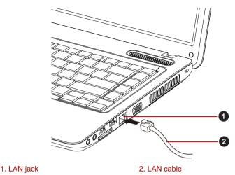
Figure 4-8 Connecting the LAN cable
