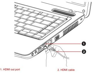
Figure 3-9 Connecting the HDMI out port
