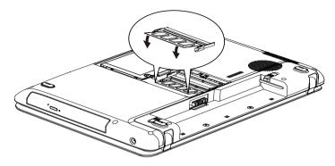
Figure 3-6 Seating the memory module-2
